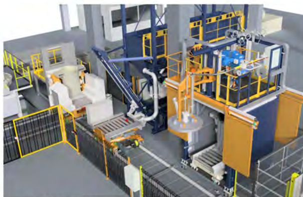
Automatic ladle transport and metallurgical treatment
