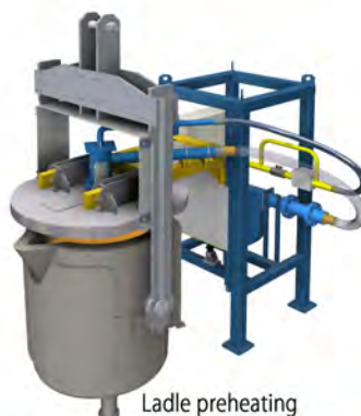
Automatic ladle transport and metallurgical treatment
